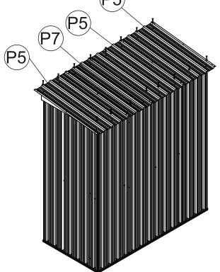
Assemble the roof flashing (15)(16)(17) with roof panels. Secure with (F1) screws with washers. Then place 4 piece of top corner(GC) on the roof joints and secure with screws with washers.
